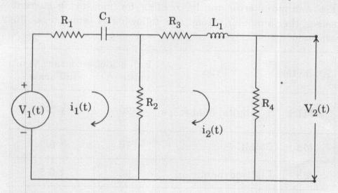
(b) The network shown below has attained steady conditions with switch K open. At t = 0, the switch K is closed. Apply Norton's theorem or Thevenin's theorem to obtain expression for current i(t) through resistor  $R_4$  given  $R_1=R_2=R_3=R_4=1.0~\Omega$ ,  $L_1=L_2=1~H$  and V=10~V DC.
